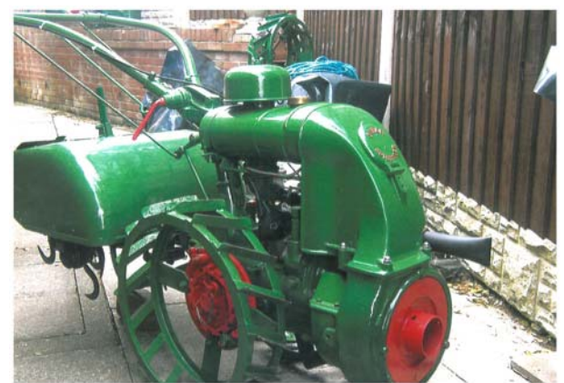
Swiss Simar Rototiller Type 50 Believed built mod 1930s, completely restored & repainted to full working order, very rare machine, single cylinder 8hp 2 stroke petrol engine, 24" rotor fitted with spring loaded tines
